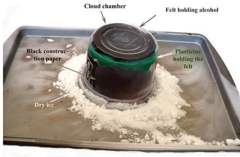
Figure 9. In your setup of the cloud chamber, the cup should be positioned upside down on the layer of crushed dry ice you made on the baking tray.
