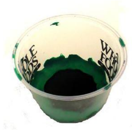
Figure 6. The first steps in preparing a cloud chamber should result in a cup whose inside bottom is covered with felt and Plasticine or clay holding the felt in place.
