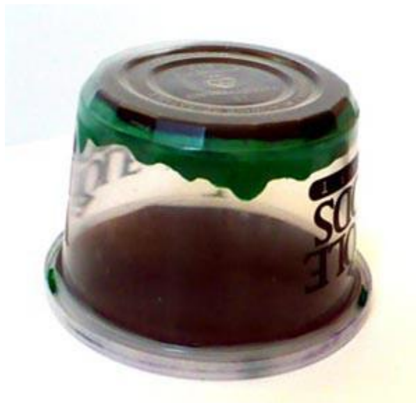
Figure 7. Picture of a cloud chamber ready to use, with the cup turned upside down, the felt held in place by the clay on the inside bottom of the cup, and the circle of black construction paper fitting inside the lid of the cup.
